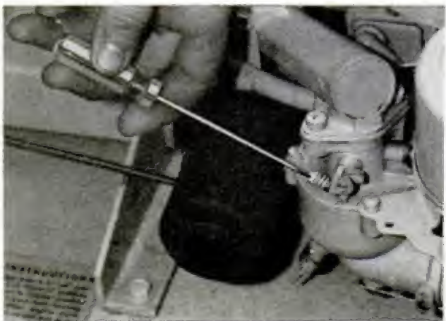
A STUCK NEEDLE VALVE can often be loosened by tapping on the carburetor bowl with a screwdriver
